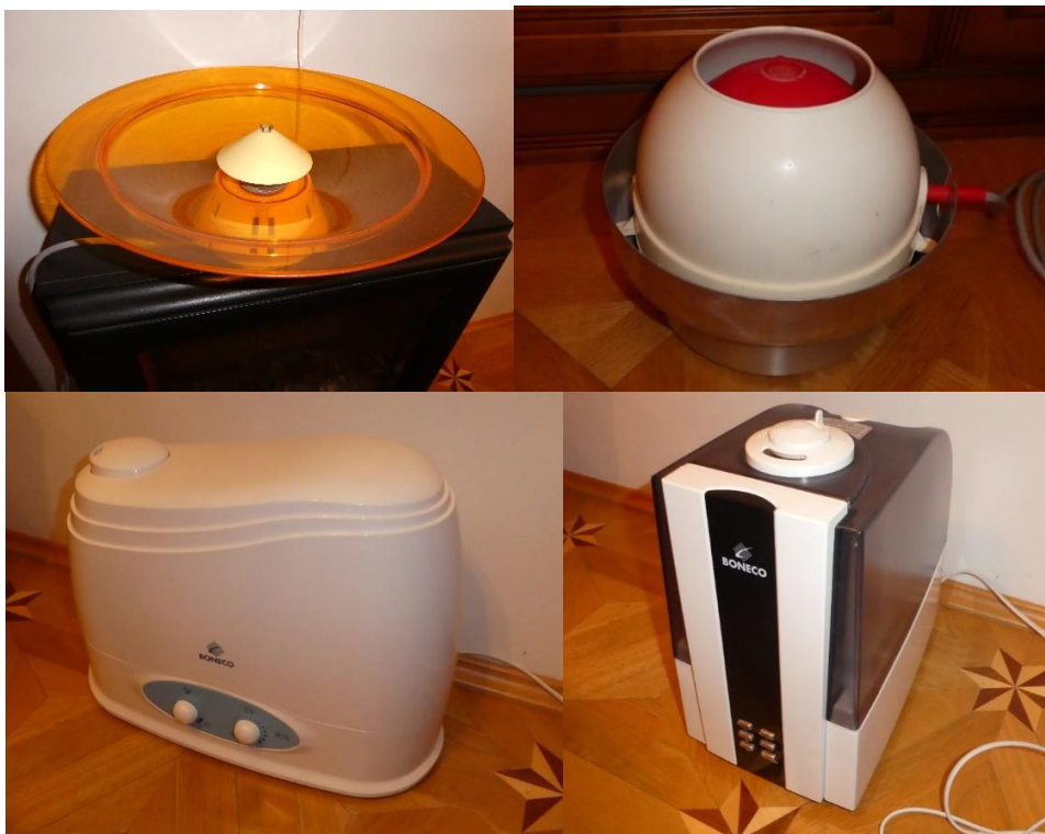
Fig. 1. Tested humidifiers: shower fountain ZV 1b (top left), humidifier with rotating disc Klad Z 15653 (top right), ultrasonic Boneco 7131 (bottom left) and automatic ultrasonic Boneco 7138 (bottom right)
